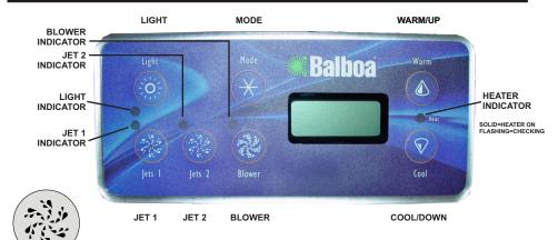
Pump 1 Key: Press this key to turn Pump 1 on and between High and Low speed. If the pump is Off the first press starts the pump in low speed and a second press turns the pump to high speed. An automatic timer turn the pump off after 30 minutes.
